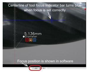
**Without the focus encoder** you will have less accurate diameter, radius and other profile measurements at lower magnifications.
