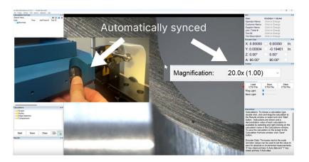
**Without the magnification encoder** the user would have to manually select the correct microscope magnification setting within the software. If the correct setting is not selected in the software the sizing on the screen will be incorrect.
