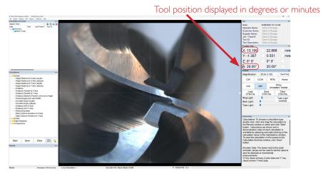
**Without the tool rotation A Axis encoder** there is a manual plunger with hard stops at -90°, 0° and 90° as well as a protractor decal. Tool position accuracy is within 1° with the manual plunger.
